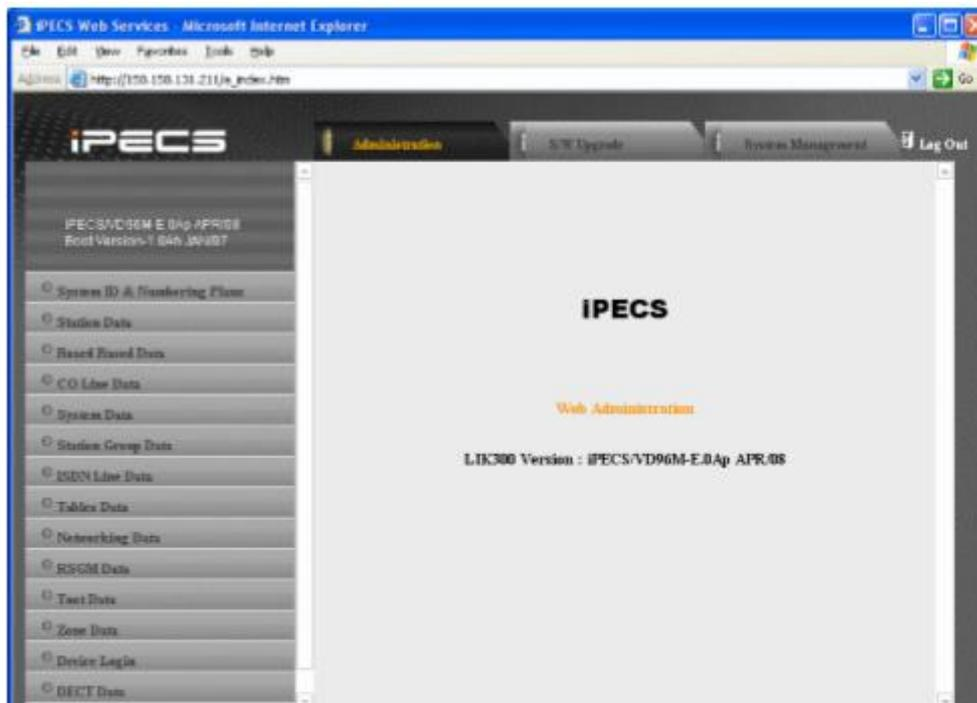
Select "System ID and Number Plan" from the list on the left. In the vacant field in the top left, enter 101 and click the "Find PGM" button. A list of devices will be displayed.
