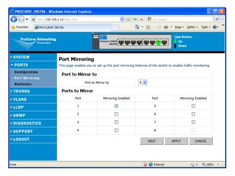
Configure with the settings;-Port to Mirror to: 8 Port 1 Mirroring Enabled: ✓
